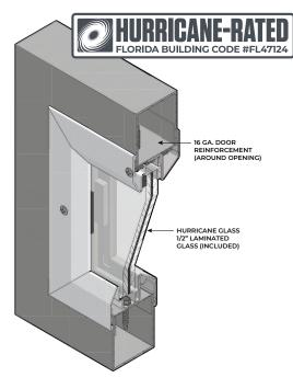
Designed for Use on Doors Manufactured Within Door Industry Tolerance of +/- ½6".
